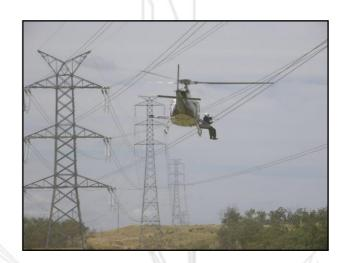
Boost Human External Cargo System – This system allows a second external cargo hook to be mounted beneath the helicopter as a redundancy hook for the safe transport of personnel. This system allows personnel to be either transported to and from towers or be able to carry out maintenance on the line whilst suspended from the helicopter.
