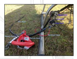
Cargo Swing & Hook — Is used for lifting underslung loads and allows the helicopter to lift loads up to 1000kg for the AS350B2 and 1200kg for the AS350B3.
