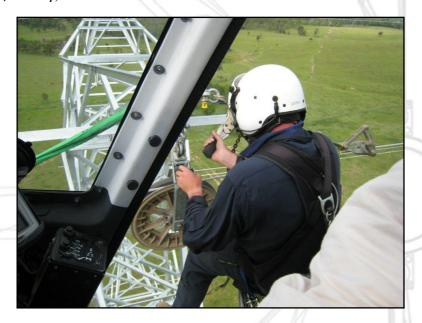
**Human External Cargo (HEC)** - Our dual hydraulic AS350B3+ is specifically equipped with the Boost Systems dual external cargo hooks for the extra security of the long line for carrying personnel.
